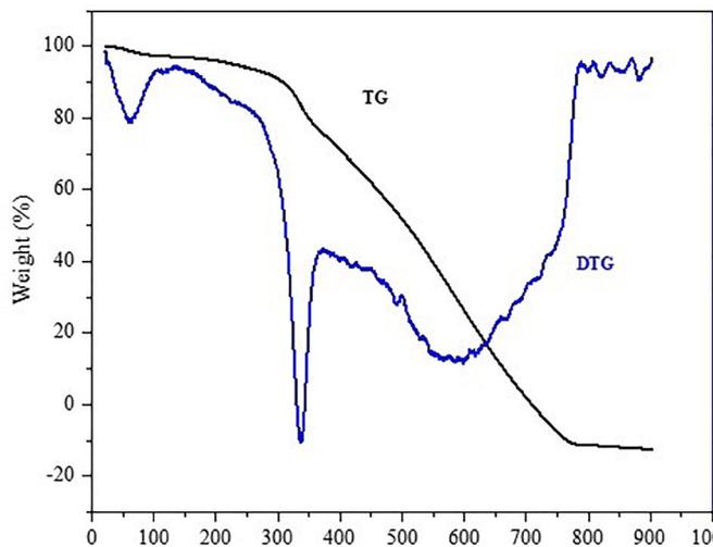
**Figure 2.** Thermogravimetric analysis (TGA) and derivative thermogravimetry (DTG) of the AWR hydrochar.
