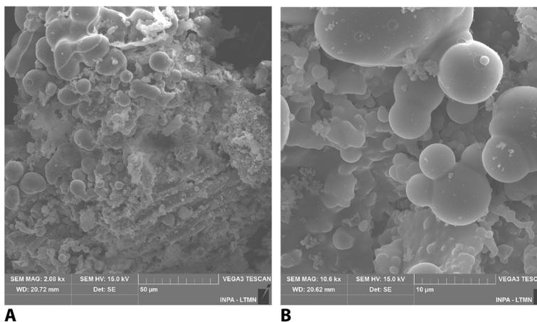
**Figure 3.** Micrographs of açai hydrochar (AWR): **A)** 2008 times; and **B)** 10600 times.
