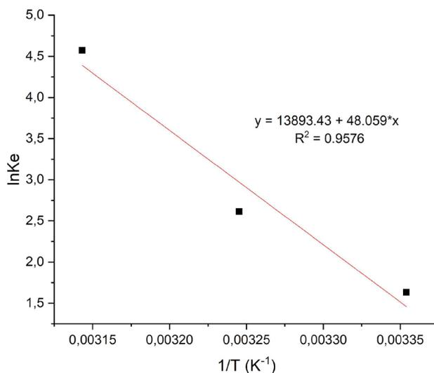
**Figure S4.** Van't Hoff plot for adsorption of Cr VI on AWR. (Conditions: *pH* = 2, *m* = 0.150 mg, and *Conc.* = 150 mg L<sup>-1</sup>, 240 min)
