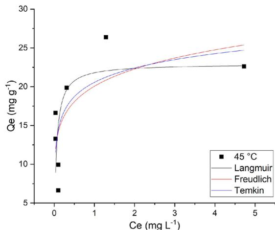
**Figure S3.** Model fit of adsorption isotherm of Cr VI adsorption onto AWR at 45 °C. (Conditions: *pH* = 2, *m* = 0.150 mg, and *Conc.* = 150 mg L<sup>-1</sup>, 240 min).
