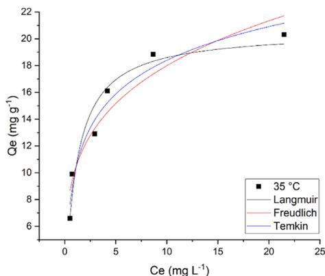
**Figure 6.** Experimental data of Cr (VI) adsorption on AWR adjusted to isotherm models at 35°C, and Model fit of adsorption isotherm of Cr (VI) adsorption onto AWR with adsorption isotherms (Conditions: pH = 2, m = 0.150 mg, and Conc. = 150 mg L<sup>-1</sup>, 240 min).
