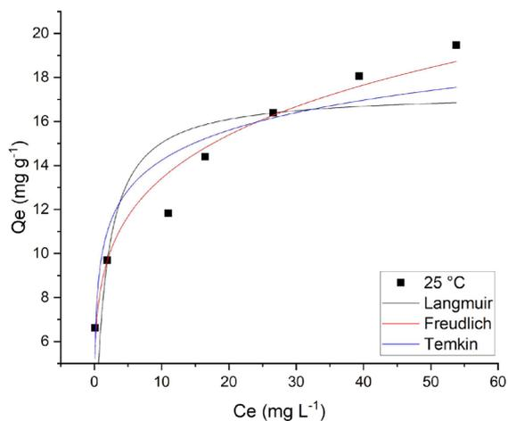
**Figure S2.** Model fit of adsorption isotherm of Cr VI adsorption onto AWR at 25 °C. (Conditions: *pH* = 2, *m* = 0.150 mg, and *Conc.* = 150 mg L<sup>-1</sup>, 240 min).
