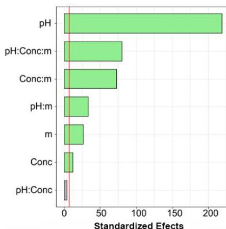
**Figure S1.** Pareto diagram for Cr (VI) removal efficiency by adsorption on AWR. Where: *m* is the mass of hydrochar (mg), and *Conc* is the concentration of Cr (VI) (mg.L<sup>-1</sup>).
