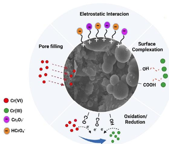
**Figure 7.** Possible mechanism of Cr (VI) adsorption by AWR.
