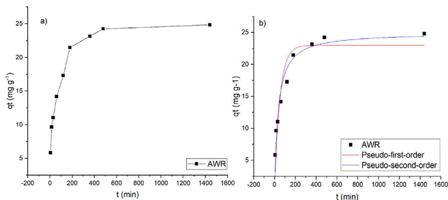
**Figure 5.** A) Experimental results for adsorption kinetics of Cr (VI) on AWR at 25°C; B) adsorption kinetics pseudo-first-order reaction model, and pseudo-second-order reaction fit model for Cr (VI) adsorption on AWR.
