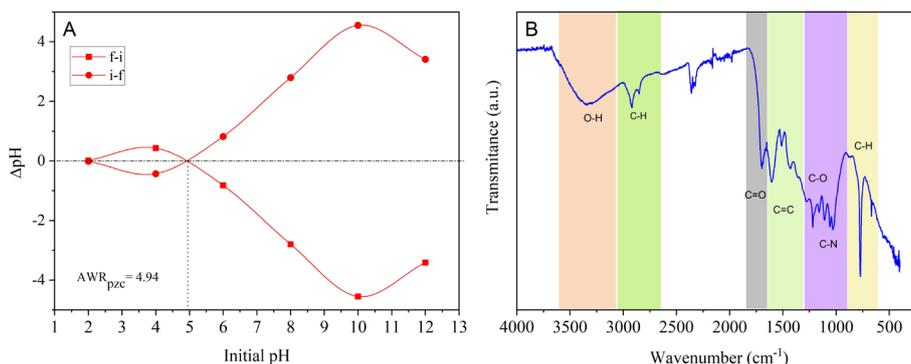
**Figure 1.** **A)** Point of zero charges ( $\text{pH}_{\text{pzc}}$ ) measured by pH variation experiments for AWR hydrochar, **B)** FTIR spectrum of the AWR hydrochar.
