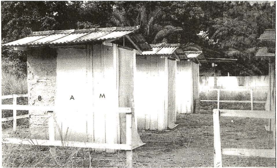
Figure 1. b= mud; a= masonry and m= wood's houses in the experimental area.
